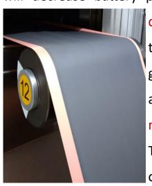
cross-web coating distribution (leading to a uniform layer thickness) are required for good battery performance (e.g. good stackability, high energy density and minimal material waste). These requirements can be fulfilled with the most advanced coating and drying technologies from FMP Technology. Our experience in this field will help us to overcome those challenges and improve your process.
